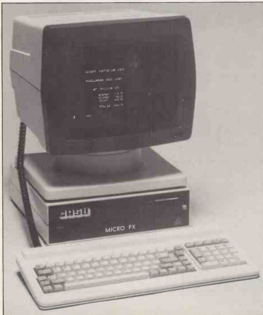
A largely British-made machine built round the 80186 CPU.
